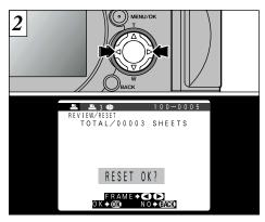
Pressing "◀" or "▶" plays back only the frames for which the number of prints has been specified, allowing you to check the settings for each frame.
